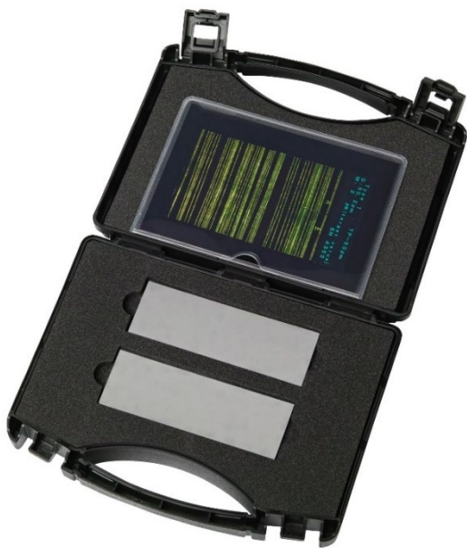
Twin Identical Panels with cracks
